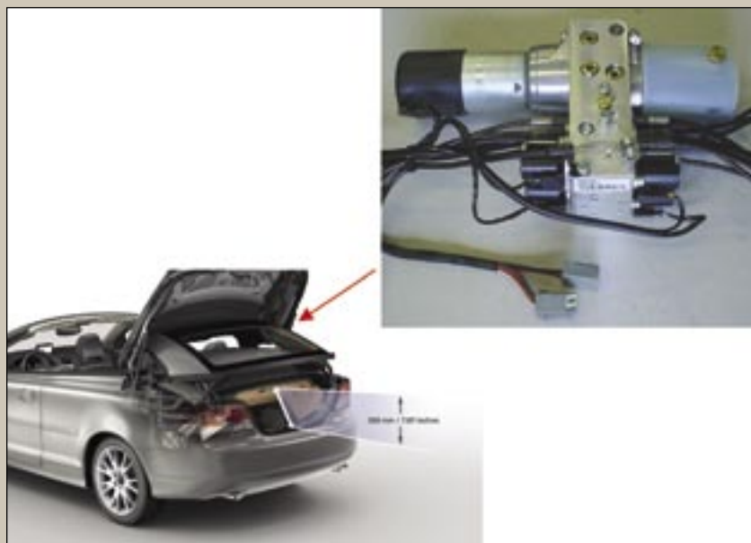
Figure 1. The Volvo C70's folding roof system produced by Webasto uses a combination of hydraulic and power electronics.
