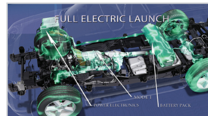
Figure 2. Unlike the 300 V battery, the dual-mode hybrid's power electronics mount under the hood.
