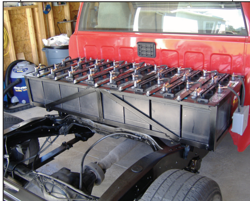
16 series-connected golf-cart batteries cradled in a center-balanced location.
