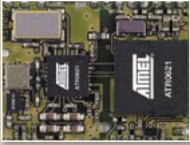
Figure 2. Atmel's ANTARIS 4 GPS chip features a CMOS baseband (ATR0621) and a BiCMOS front end (ATR0601).
