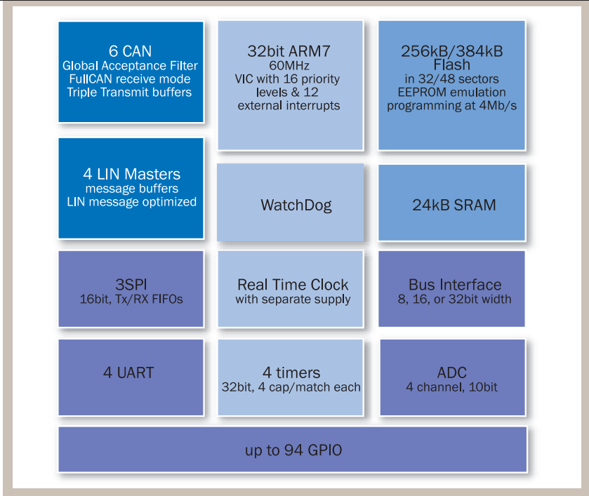
Figure 2. Offering both CAN and LIN gateway functionalities, Philips' SJA2020 is designed to replace multiple eight-bit MCUs in body-control applications with a single 32-bit device.
